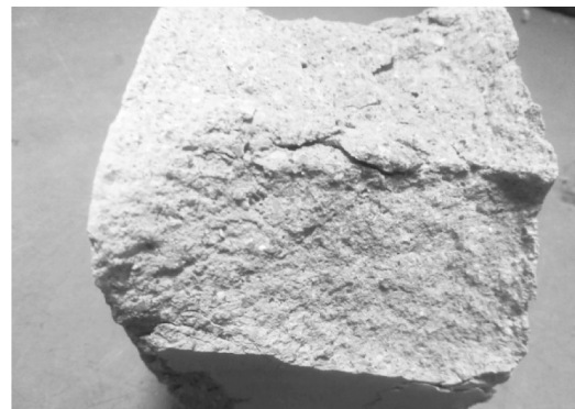
图1 受压破坏后的试件 Fig.1 Test piece after pressure damage
