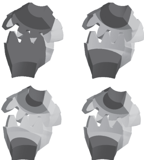
图 8 锥齿轮副齿面接触应力变形 Fig.8 Deformation of gear contact stresses
