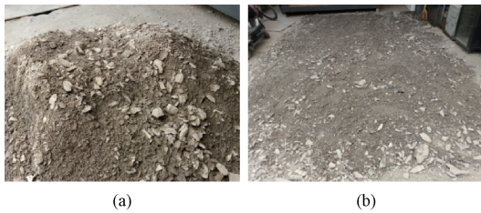
图 1 TBM 洞挖料 Fig.1 TBM hole excavated material
