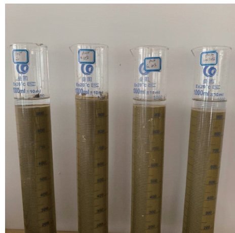
图6 掺入不同外加剂泥浆稳定性对比 Fig. 6 Stability comparison of mud mixed with different additives
