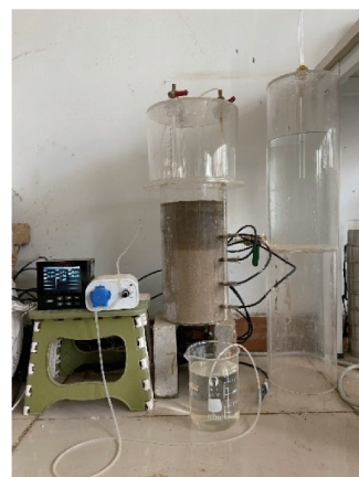
Fig. 1 Rain infiltration test instrument diagram
