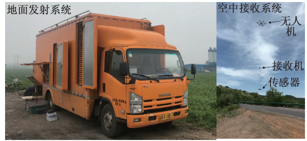
图 2 JL-GAEM 地空频率域电磁探测系统实物图 Fig. 2 JL-GAEM ground airborne frequency-domain electromagnetic system
