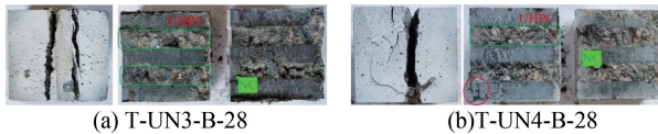
图7 UHPC-NC 劈裂拉伸破坏模式:NC强度的影响 Fig. 7 Splitting tensile failure pattern of UHPC-NC specimen: effects of NC strength
